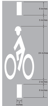
Figure 3: Bicycle detection stencil (2009 MUTCD Figure 9C-7)
