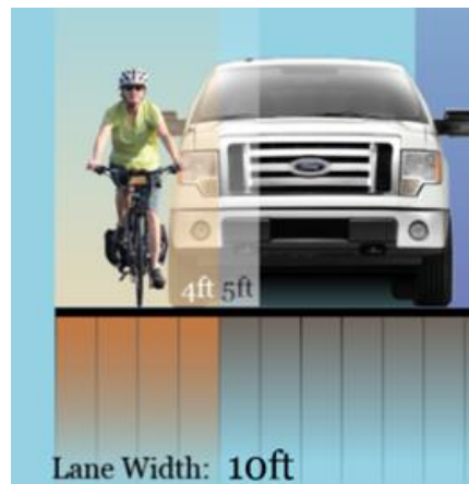
Figure 12: Scale drawing of a bicyclist and a pickup truck in a 10' wide lane. A bicyclist needs about four feet of operating space to maintain balance. There isn't enough room for a motorist to pass a bicyclist within the lane without risking a collision. [Graphic by Keri Caffrey]
