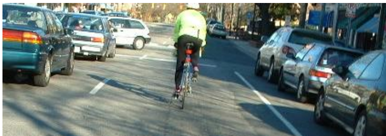
Figure 14: Controlling a travel lane by riding near its center deters unsafe same-lane passing and makes a bicyclist more visible to other drivers.
