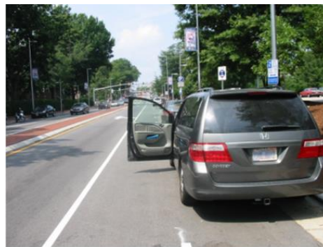
Figure 16: To avoid the danger of being struck or startled by opening car doors on this street, a bicyclist must operate left of the solid white line.
