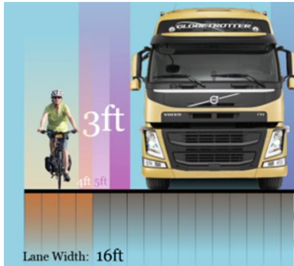
Figure 13: A minimum of 16 feet is required for safe same-lane passing of a bicyclist by a truck, transit bus, or landscaping trailer. [Graphic by Keri Caffrey]
